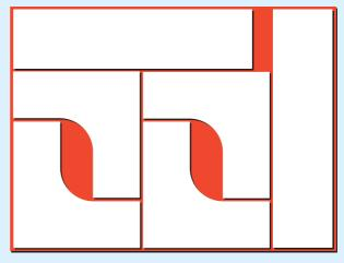
to process 7 kitchens using the 1220x2440 sheets. The machining of the eighth kitchen is effectively free. Add to this the savings from better yield that the larger sheet will give you and the savings in labour, and you will realise an increase in production and a saving in associated costs.
