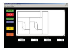
The operator panels within the user interface are tailored to suit each installation Genuine industry standard G-Code programming language means the end user can choose machining software that best suits their application. Commonly used software packages used in the joinery
