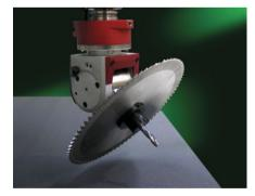
Aggregates available include horizontal drilling and routing units, sawing units, corner notching and floating head units.
