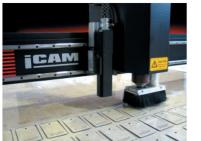
iCAM Ultima Machine was built to process aluminium. This machine features a misting unit for cooling and T-Slot Table for part clamping as well as a custom clamping system to hold aluminium extrusions while processing. Process size 2050mm x 6100mm.
