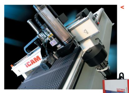
iCAM Ultima incorporating saw for processing across the Y axis and 7.5hp spindle with 10 station auto tool change unit. This machine was built to process Phenolic panel and features a custom matrix table top to allow proccessing of the underside of the edge of the panel. Process size 1525x6000m.
